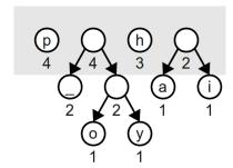
Note when we build a combined node, it doesn't represent a character like the leaf nodes do. These *interior nodes* are used along the paths that eventually lead to valid encodings, but the prefix itself does not encode a character.
