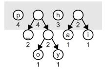
Again, we pull out the two smallest nodes and build a tree of weight 4:
