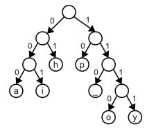
The path to 'h' is just left right or 01, the path to 'y' is right-right-right or 1111. Notice that the prefix property of the Huffman encoding is visually represented by the fact that characters only occupy leaf nodes (i.e. those nodes which are not a prefix of any further nodes).
