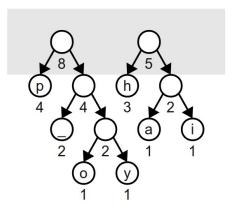
And finally, we combine the last two to get our final tree. The root node of the final tree will always have a weight equal to the number of characters in the input file.
